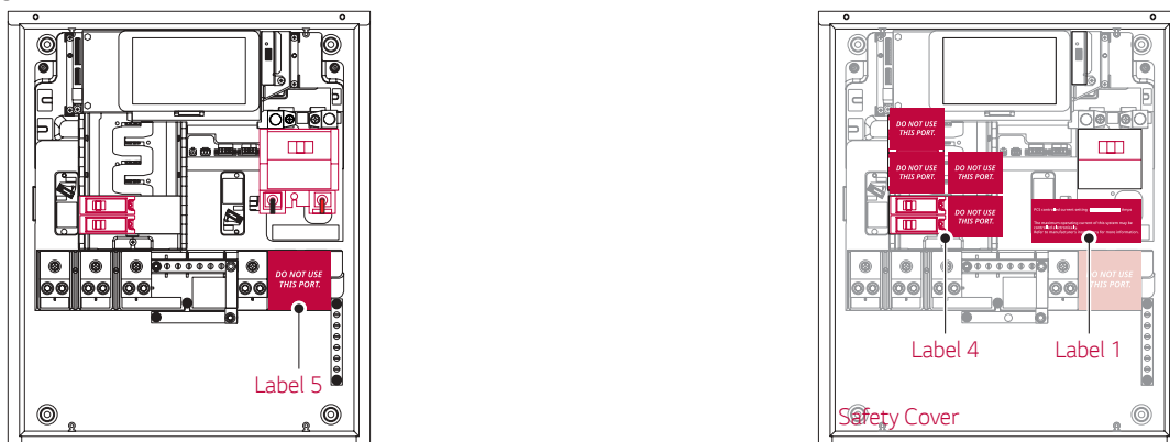
< Figure 6. Circuit Breakers Installation & Label Positions : PV+ESS Combiner connected to SE Box thru BJ series breaker >
