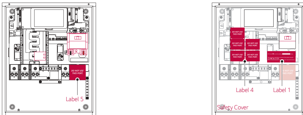
< Figure 5. Circuit Breakers Installation & Label Positions : PV+ESS Combiner connected to SE Box thru Terminal Block >
